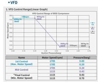
• VFD + RECYCLE VALVE : VFD(50 ~ 100%), RECYCLE VALVE(0~50%)
