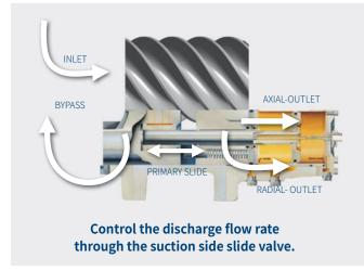
• SLIDE VALVE + RECYCLE VALVE : SLIDE VALVE(10 ~ 100%), RECYCLE VALVE(0~10%)
